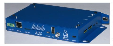
The A2X has been designed from the ground up to be a compact, fully-featured 2-way capable ALERT2 IND. Measuring just 7.5" x 4", the A2X is much smaller than our
